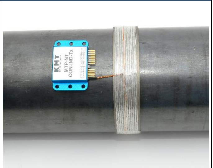
Twist the flexible wire and solder it on the MTP-NT IND-Tx (isolate all solder points with shrink tubing)
