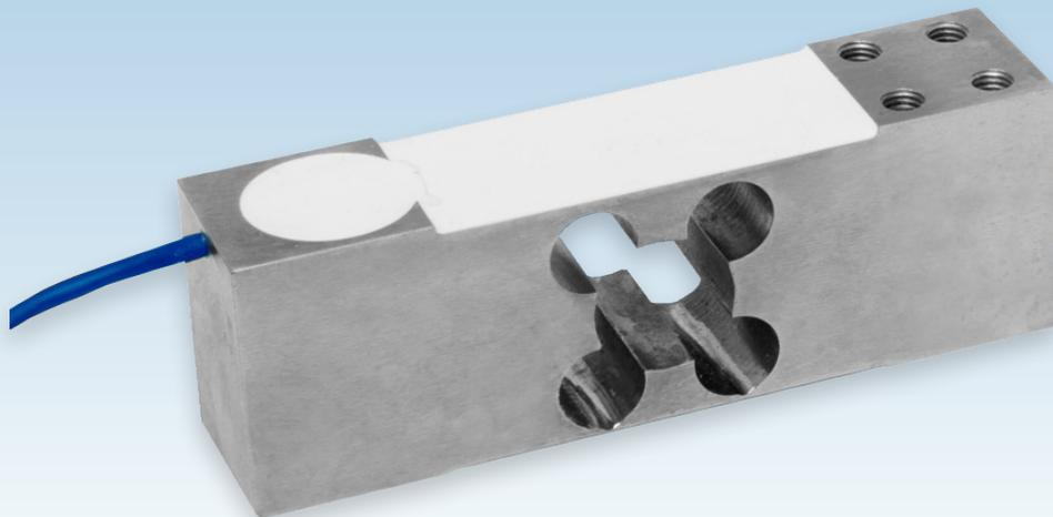
The T12A double bending beam single point load cell is ideal for high accuracy weight measurement with off-centre loads when the environment does not require stainless steel. Its nickel plated alloy steel construction, with silicone sealing to IP66, provides a cost-effective solution that is approved to 4000 divisions OIML R60 Class C. As standard, the T12A is supplied with a screened polyurethane cable; this provides a higher level of resistance to cuts and damage than a PVC cable.
