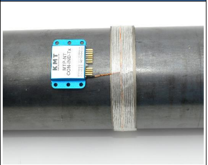
Twisted also the flexible wire and solder it on the MTP-NT IND-Tx (isolate all solder points with shrink tubing)
