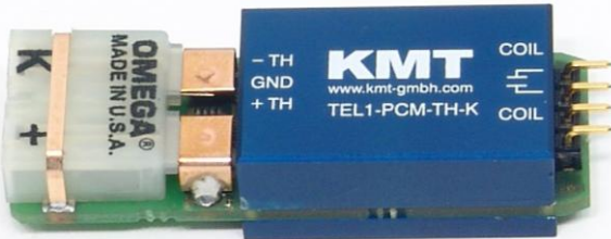
with female K type thermocouple connector
